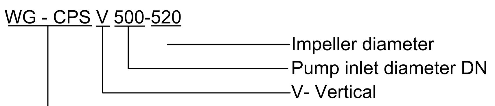
(H-Petrochemical-high temperature-derived) High efficiency double-suction centrifugal Pump —Split case pump
